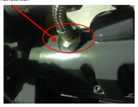
2. COALTRAM owners with the old pump solenoid coil may choose to continue using old pump solenoid coil and regularly monitor for any oil ingress as per Safety Bulletin SB14001 or replace with new pump solenoid coil. Vehicles fitted with the new style pump solenoid coil may continue running without modification.
