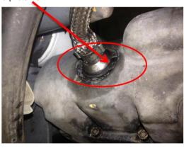
New coil with nut retention
