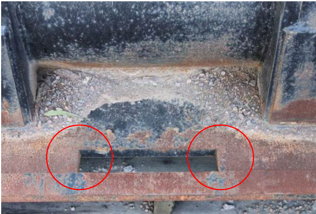
Figure 1: Inspect all welds and plates for indications of cracks and signs of damage, deterioration and wear. Pay particular attention to engagement retention areas and tongue engagement position.
