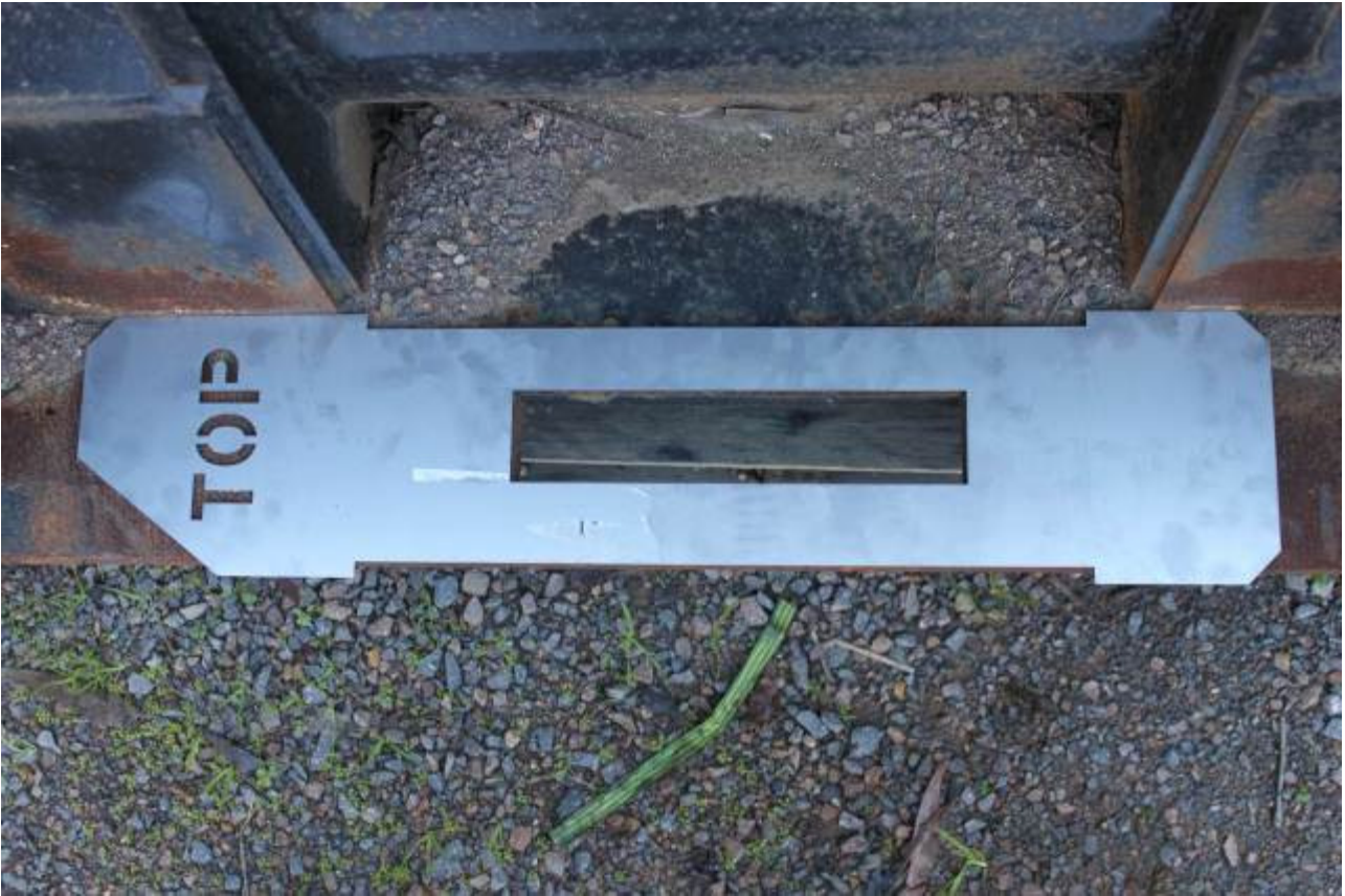
Figure 3: Implement Inspection Gauge Part No. 5-12170701 can also be used to assess for wear to the QICS tongue engagement location.
