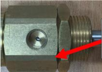
Non-conforming unit. No serial no. in this location, Smaller orifice, No grub screws.
