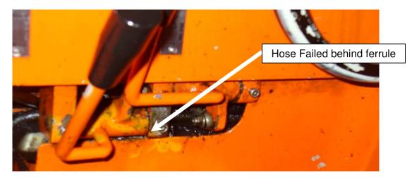
The hose was replaced with a hose fitted with suppression sleeving as per the Colliery standard. The hose failure is shown below.
