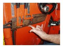
Identified in this incident was the potential for any exposed joystick hoses to generate a similar incident. To prevent this it is recommended to fit the cover shown below. Part no. 0508-50043.
