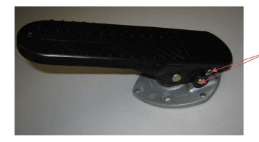
Remove original split pin and pivot pin
