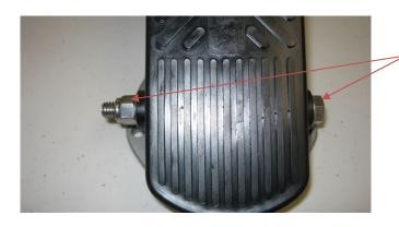
Install 3/8 x 4 ½ inch stainless steel bolt, nyloc nut and washers
