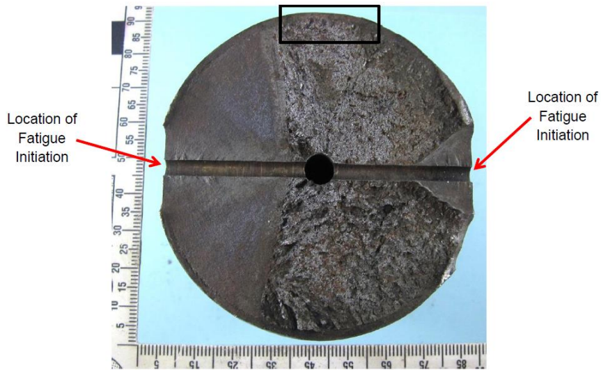
Figure 2: Fracture face of broken pin
