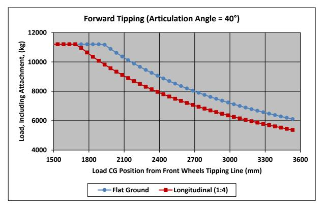
The maximum limit load including attachment is 11200 kg
