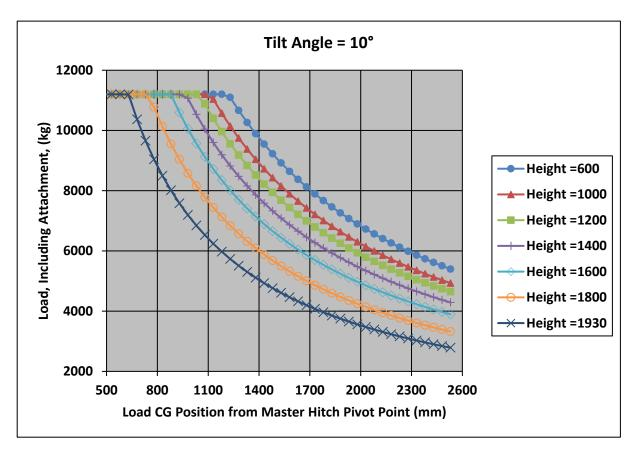
The maximum limit load inc, attachment is 11200 kg
