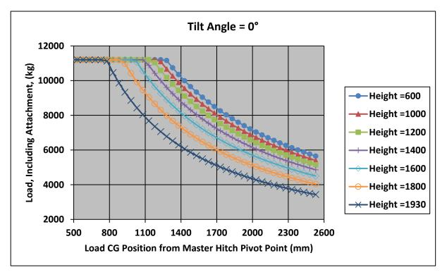
The maximum limit load including attachment is 11200 kg
