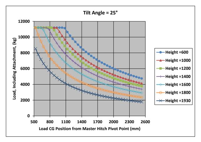
The maximum limit load including attachment is 11200 kg
