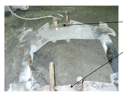
As can be see from this photo the top end of the bolster appears to have some compression marks on the face between the differential and the bolster, while the bottom end only had loose dirt sitting on the faces indicating no compression between the faces.
