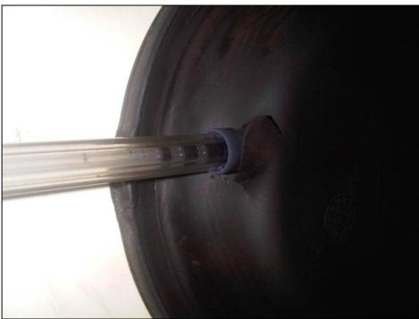
Based on the age of the machine, the estimated diaphragm component life was 8 years. This was the first known occurrence of a diaphragm failure on a VLIDD machine. Based on the information and evidence received, it was not possible to identify the root cause of the diaphragm failure.
