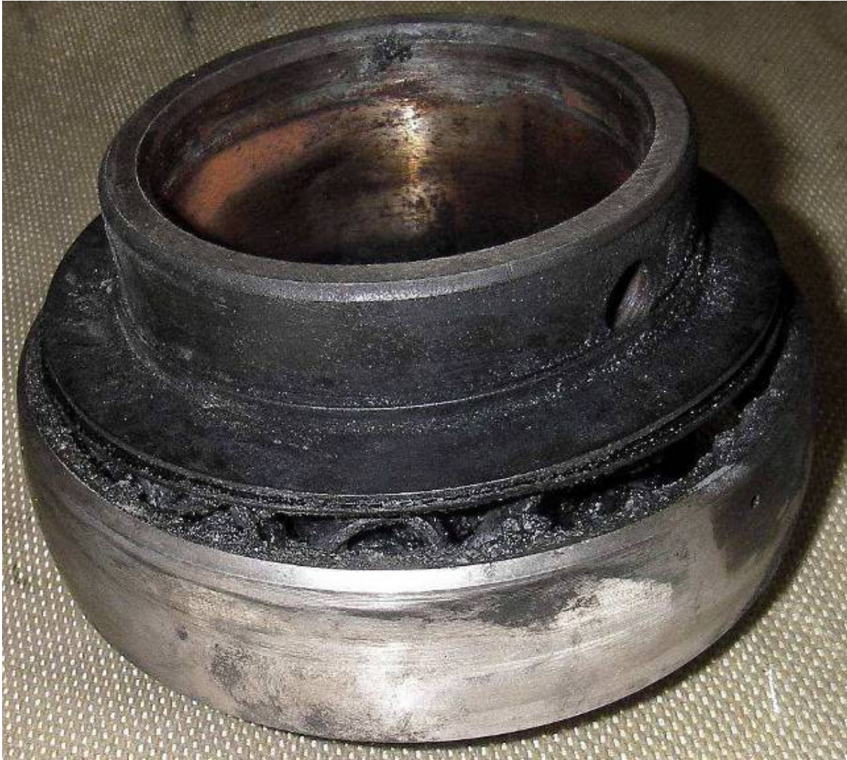
Figure 2 Ball roller bearing in the as received condition (before cleaning)
