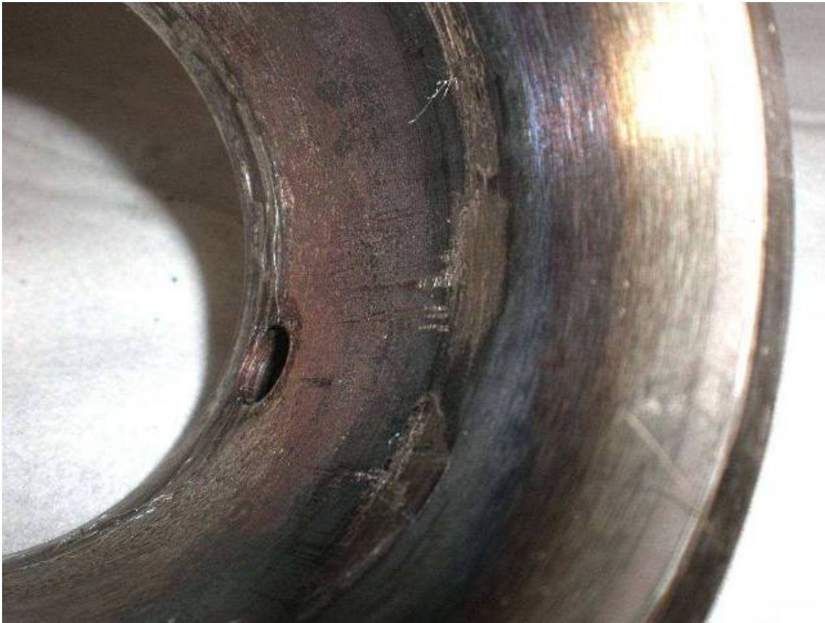
Figure 11 View of the damage caused by the driveshaft
