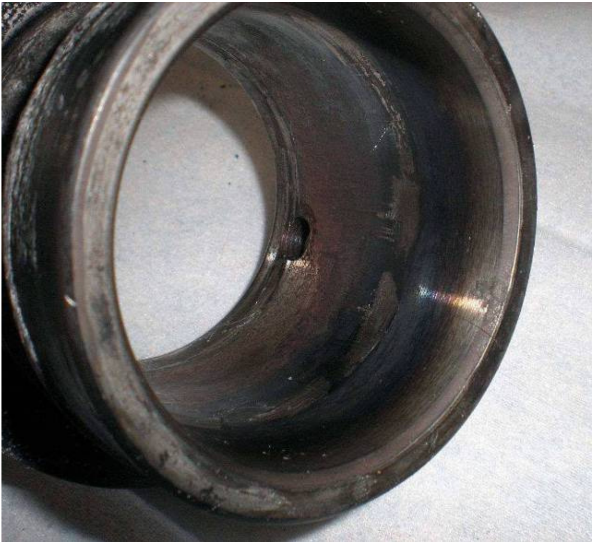
Figure 9 Close up view of the outer raceway spalling
