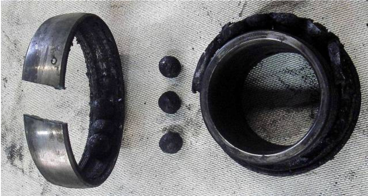
Figure 4 Bearing after removal of the outer raceway
