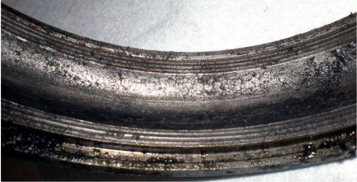
Figure 9 Close up view of the outer raceway spalling
