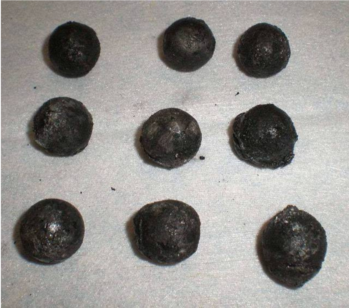
Figure 7 View of the ball rollers; note the severe deformation present in some of the balls
