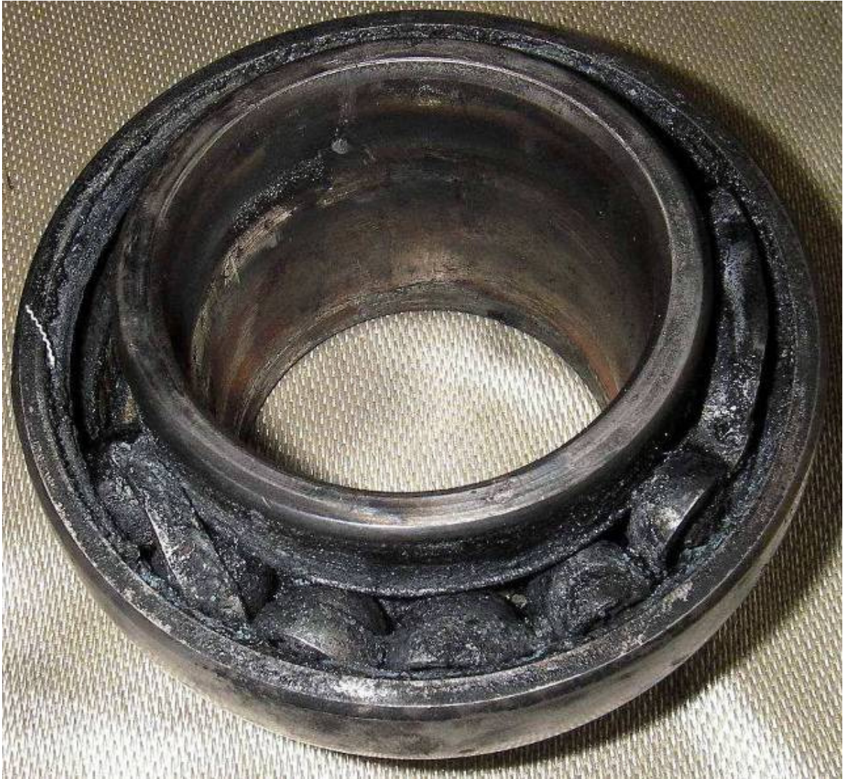
Figure 1 Ball roller bearing in the as received condition (before cleaning)
