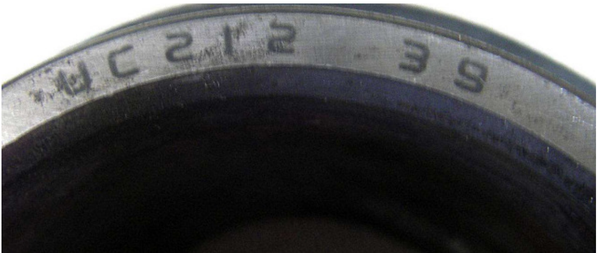
Figure 3 Identity number on inner raceway
