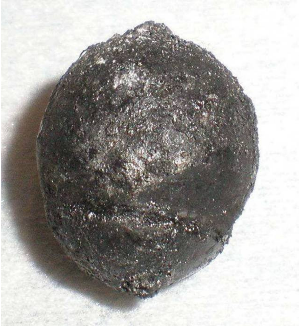
Figure 8 Close up view of a discoloured and deformed roller ball
