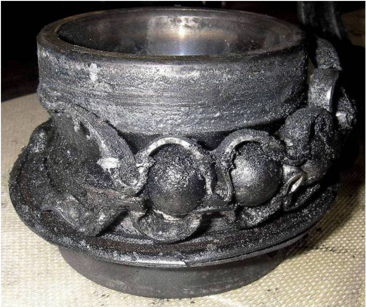
Figure 5 Close up of the bearing without the outer raceway
