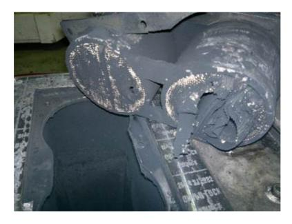
Figure 2: Exhaust Purifier Element Deformation / Damage
