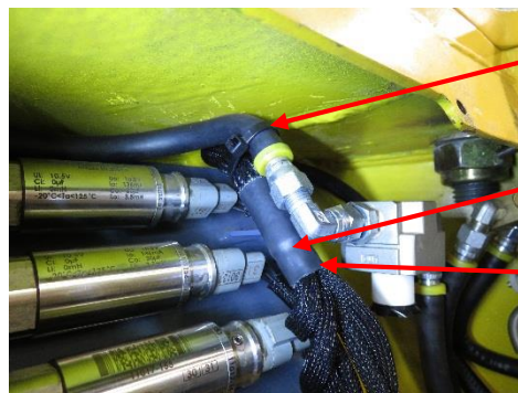
Figure 4: Cable Tied in Place With Over-molding Verticle
