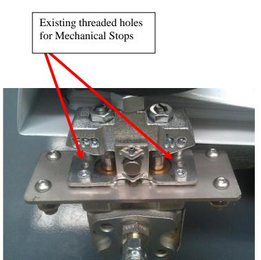
Standard Stick Steer Lever (No Mechanical Stops Fitted)
