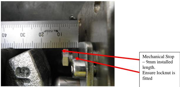
Modified Stick Steer Lever (Mechanical Stop Fitted)
