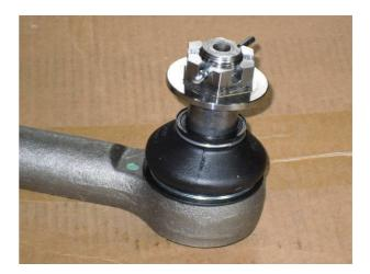
Flanged nut fitted to a new ball joint/ tie rod
