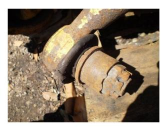
Flanged bush still fitted to the ball joint
