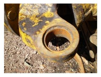
Machined recess in steering arm
