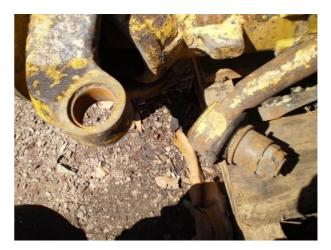
Dislocated left hand side steering arm and tie rod linkage.
