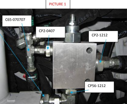
Hose up the pressure reducing valve as per picture 2.
