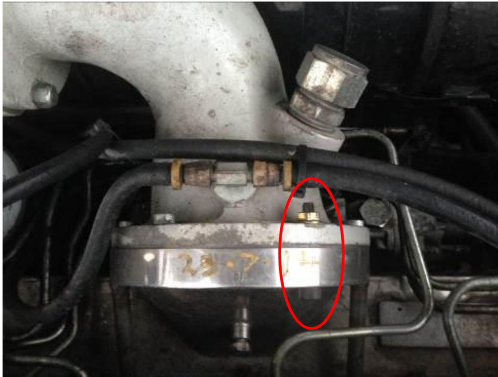
Figure 4: Photograph showing an example of the use of a through bolt fastener (as installed to a V3 engine configuration).
