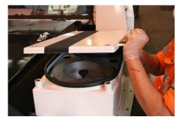
5. Unscrew retaining knobs & remove filter retaining caps.
