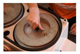
8. Inspect condition of seal and ensure in serviceable condition. Carefully lower & secure lid using retainers.
