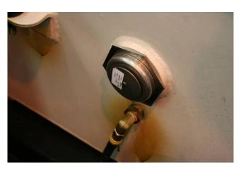
The water tank is pressurised to ensure the Exhaust Conditioner has constant water supply with a pressure release cap fitted to relieve excess pressure. Filling of the water tank is carried out via the cap, located in the top of the tank.
