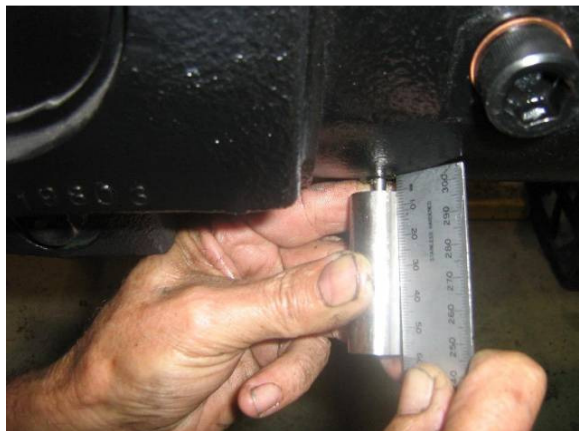
Figure 7. Tool at 5mm protrusion indicates medium wear.
