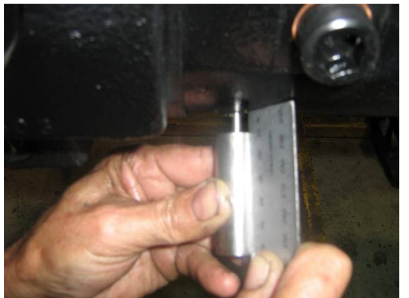
Figure 8. Tool at >5mm protrusion indicates high wear. Brake replacement required.
