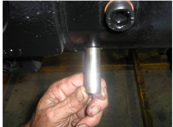
Figure 6. Brake wear check tool fully inserted indicates low brake wear.
