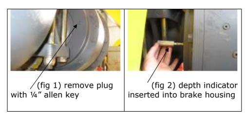
7. Depth gauge should read in area between wear limit range
