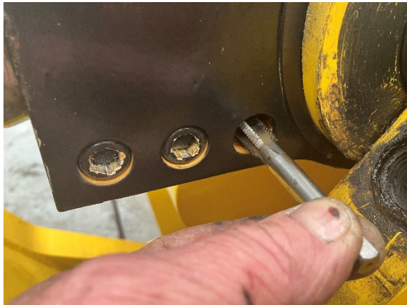
Figure 6. Clean No.1 bolt hole with M12 x 1.75 thread tap.
