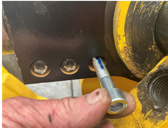
Figure 7. Install new bolt M12 x 1.75 x 60 Grade 12.9 with Loctite 243 applied to the thread.
