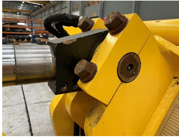
Figure 2. Inspect security of clevis against rod end shoulder.
