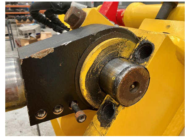
Figure 5. No.1 clamp bolt removed.
