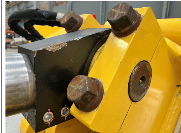
Figure 11. Replace cylinder pin end cap and torque retaining bolts to 1480 Nm whilst maintaining an even clamp gap.
