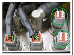
Figure 12 – fitted Blanking Plugs
