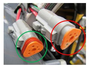
Figure 1 - Missing Seal
