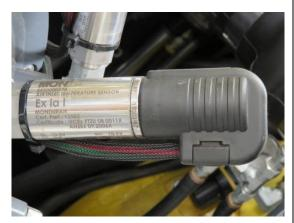
Figure 13 - Sensor Weather Boot
