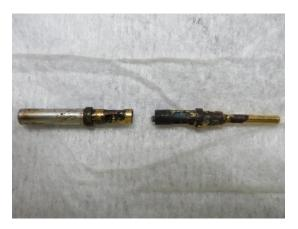
Figure 5 - Corrosion
