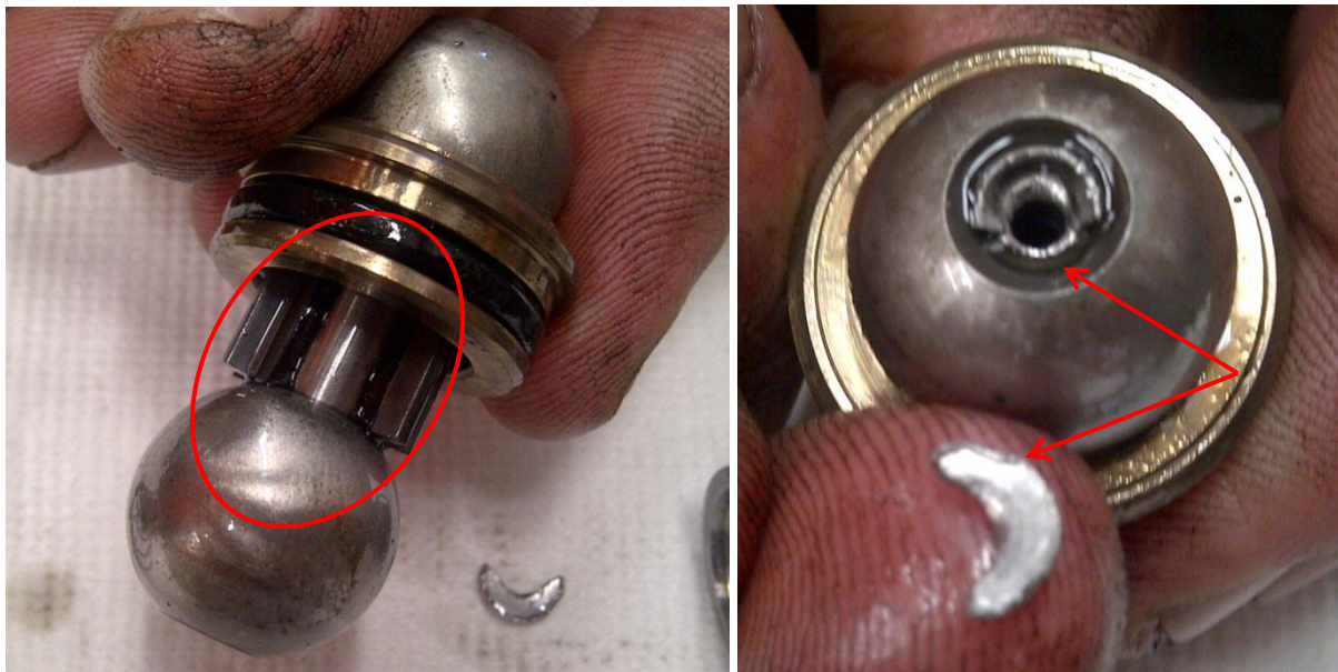
Figure 2: Photographs showing the porting valve from the recent service brake valve failure in 2013, highlighting the missing piece of spline and the fractured metal from one of the swaged ball ends.
