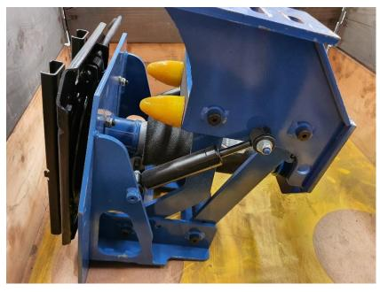
Figure 1 - Jel seat assembly - PPK Part Number 5520009577
