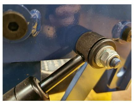
Figure 2 - Jel seat dampener rod-end to bush housing
