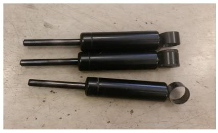
Figure 3 – Jel dampeners with rod-end to bush housing weld failure
