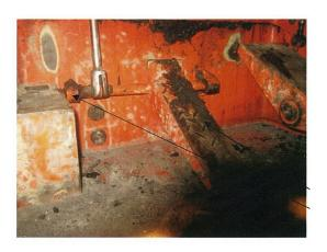
Brake pedal assembly- arrow points to broken pivot boss on brake pedal.
