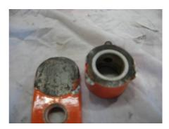
Detail of broken pivot boss showing only two "tack" welds with no weld penetration.
