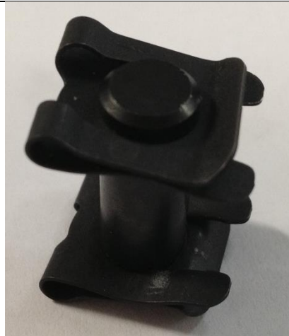
Figure 3: New retaining clips installed on pin
