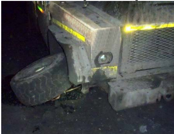
Photo 1: Failure to front right-hand steering knuckle
