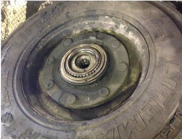
Photo 3: Failure to stub axle left-hand side
