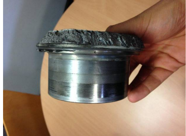
Photo 6: Failed stub axle
