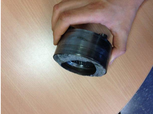
Photo 5: Stub axle re-sleeved
