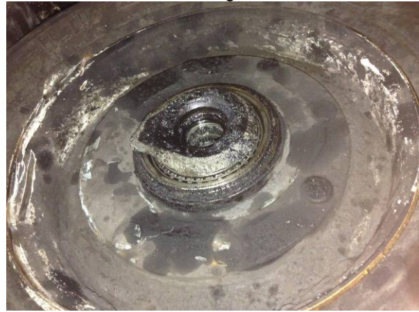
Photo 4: Failed stub axle right-hand side
