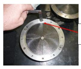
Feeler gauge inserted into gap as shown. Measurements to be made at multiple positions around Housing-Element circumference.
