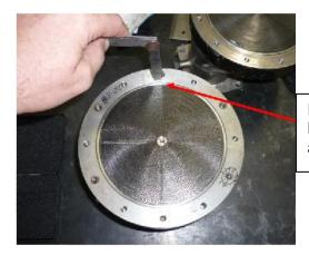
Feeler gauge inserted into gap as shown. Measurements to be made at multiple positions around Housing-Element circumference. Specified Gap 0.4mm Maximum
