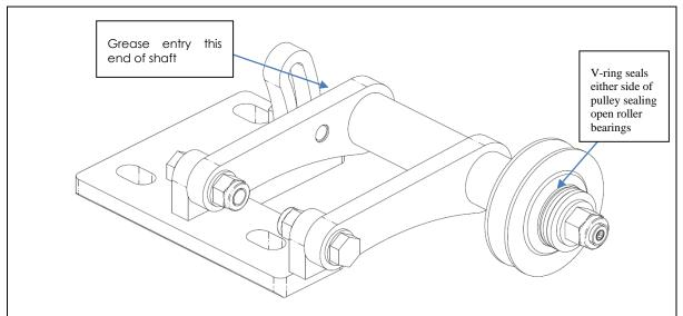
Figure 2: New greasable idler pulley
