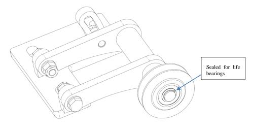
Figure 1: Original idler pulley
