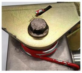
Figure 4: New spring larger coil diameter (almost lines up with edge of pedal)
