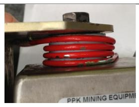
Figure 2: New spring with 3 coils (4 visible strands)
