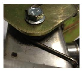
Figure 3: Old spring - small diameter coil (does not extend out to edge of pedal)
