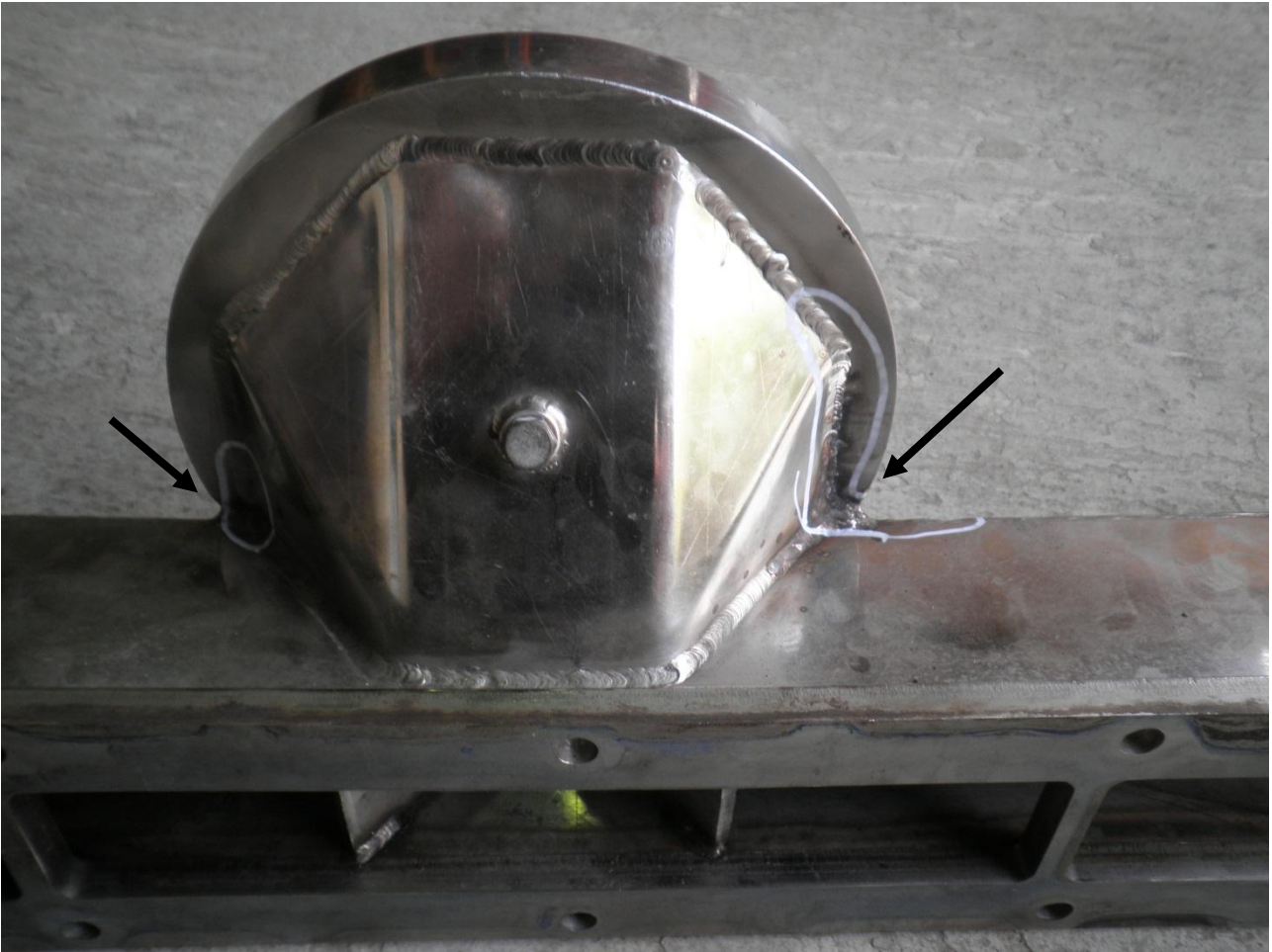
Figure 1: Photographs showing a JUG-A-0 air inlet manifold, highlighting the location at which fatigue cracks have been identified.
