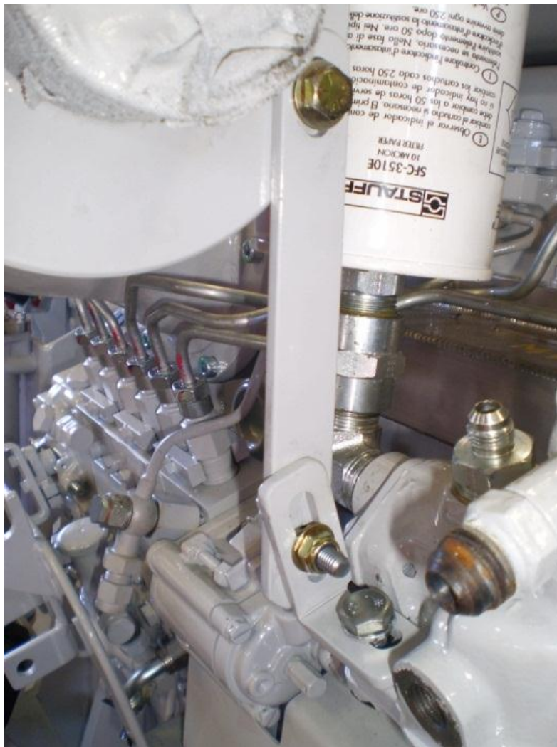
Figure 2: Photograph showing the support bracket (Part No. 0508-60081) for the air inlet ducting and strangler valve assembly for V3 machines (machines with gear driven superchargers), as installed.
