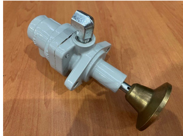
Park brake valve with open flow breather installed, a cut-off 90 degree fitting.
