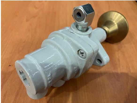
Park brake valve with open flow breather installed, a cut-off 90 degree fitting.
