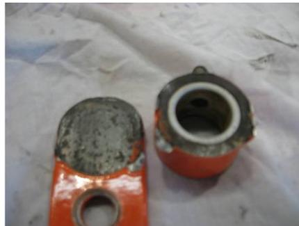
*Detail of broken pivot boss showing only two "tack" welds with no weld penetration.*
