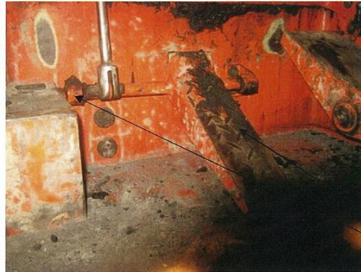
*Brake pedal assembly- arrow points to broken pivot boss on brake pedal.*
