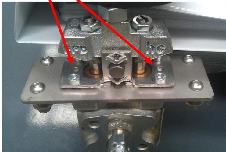
*Standard Stick Steer Lever (No Mechanical Stops Fitted)*
