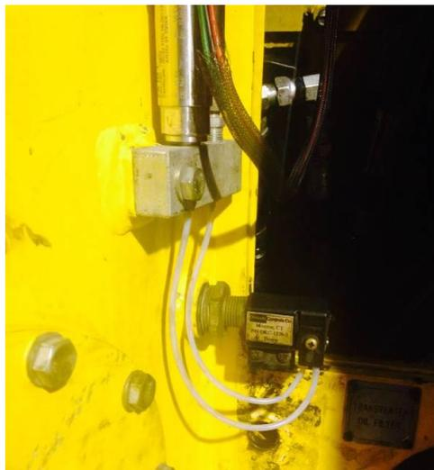
*Figure 1: PTFE tubing installed*
