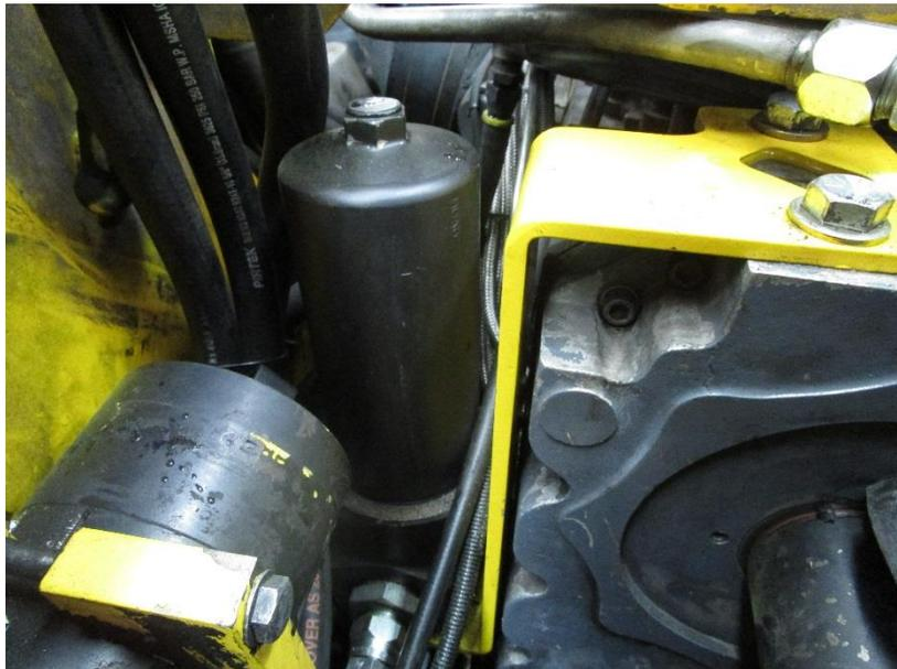
*Figure 1: Steer filter mounted on side of upbox*
