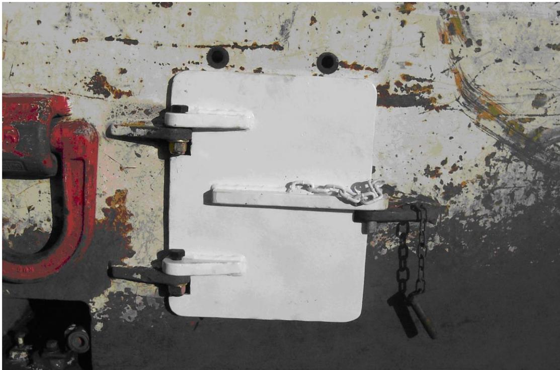
**New design fitted cover over the scrubber float cam mechanism**
