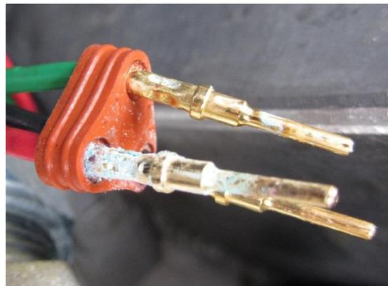
**Figure 6 - Corrosion and Contamination**
