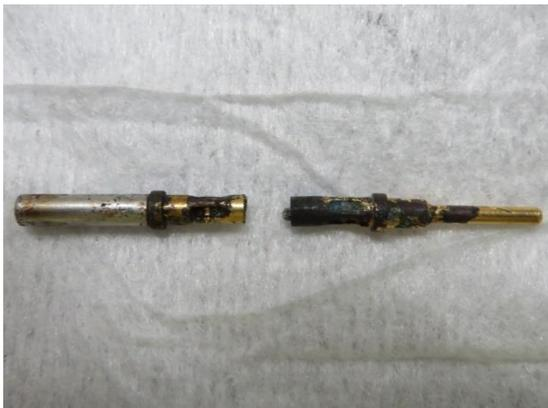
**Figure 5 - Corrosion**
