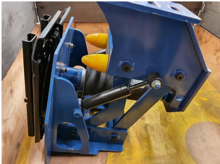
Figure 1 - Jel seat assembly - PPK Part Number 5520009577
