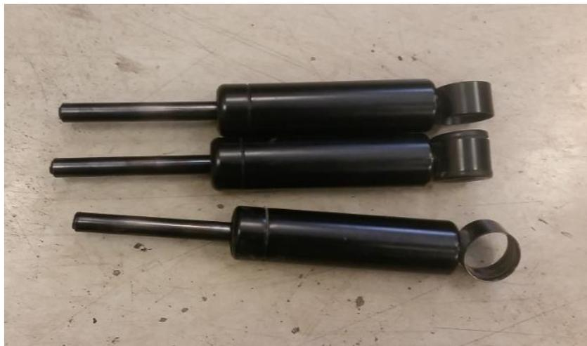
*Figure 3 – Jel dampeners with rod-end to bush housing weld failure*
