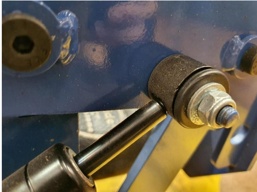
*Figure 2 - Jel seat dampener rod-end to bush housing*
